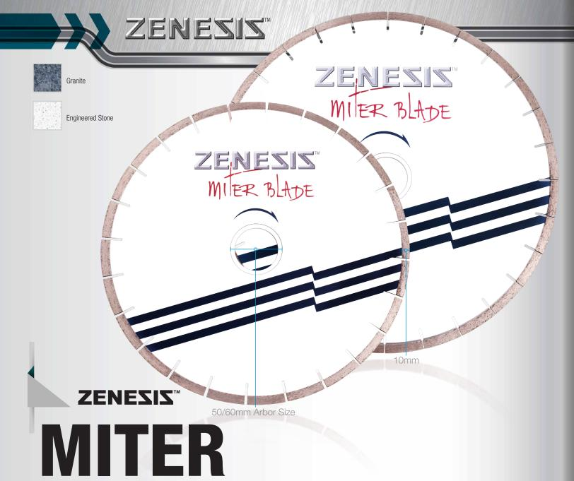
The ZENESIS<sup>TM</sup> MITER blade is specifically designed to deal with the added side stress put on blades when miter cutting. Most mega segment (over 20mm) blades are designed only for straight cutting. The added downward pressure put on these blades while miter cutting can cause flexing at the weld and premature tension loss in the core. Our 10mm segments do not flex at the weld which makes it the straightest cutting miter blade on the market.
